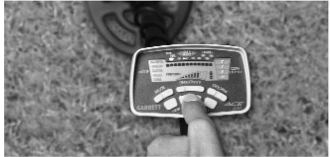
distance between the coil and the ground remains constant throughout the entire pinpointing process; in this case, that distance is zero inches. If the ground's terrain does not allow for this type of "coil scrubbing" then do your best to maintain constant separation between the coil and the ground.
